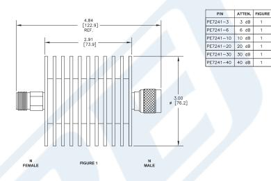
3 dB Fixed Attenuator, N Male To N Female Black Anodized Aluminum Heatsink Body Rated To 100 Watts Up To 4 GHz from Pasternack Enterprises has same day shipment for domestic and International orders. Our RF, microwave and millimeter wave products maintain a 99% availability and are part of the broadest selection in the industry.
