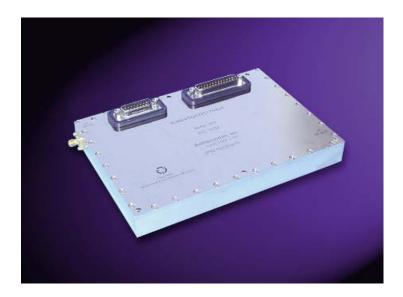
compact module. Standard housing size is approximately 5.0 X 7.0 X 1.0 inches. SMA female connectors are standard in the RF input and output ports. DC, command/control and telemetry signals are accessible through two D type subminiature connectors. Housing is environmentally sealed.
