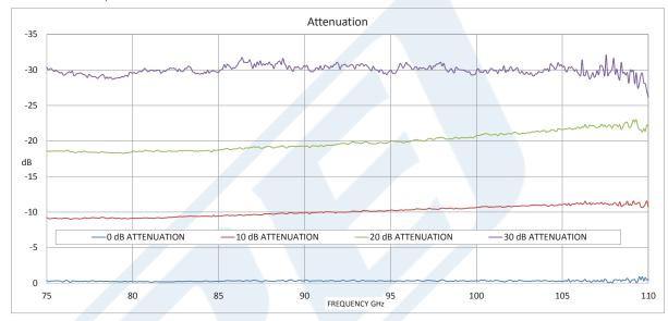
0 to 30 dB Waveguide Continuously Variable Attenuator, WR-10, From 75 GHz To 110 GHz, UG 387/U-Mod Flange from Pasternack Enterprises has same day shipment for domestic and International orders. Our RF, microwave and millimeter wave products maintain a 99% availability and are part of the broadest selection in the industry.
