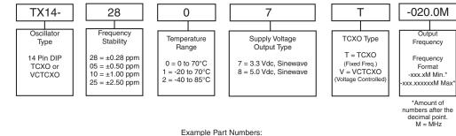
TX14-2807T-020.0M = 14 Pin DIP package, ±0.28 ppm, 0 to 70°C, 3.3 Vdc, Sinewave Output, TCXO, Output Frequency 20.0 MHz TX14-0528V-38.88M = 14 Pin DIP package, ±0.50 ppm, -40 to 85°C, 5.0 Vdc, Sinewave Output, VCTCXO, 38.88 MHz
