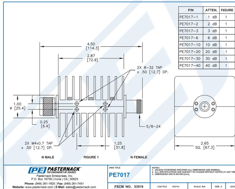
10 dB Fixed Attenuator, N Male To N Female Black Anodized Aluminum Heatsink Body Rated To 25 Watts Up To 18 GHz from Pasternack Enterprises has same day shipment for domestic and International orders. Our RF, microwave and millimeter wave products maintain a 99% availability and are part of the broadest selection in the industry.
