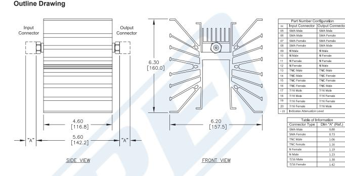
30 dB Fixed Attenuator, 7/16 DIN Female To 7/16 DIN Male Directional Black Aluminum Heatsink Body Rated To 300 Watts Up To 3 GHz from Pasternack Enterprises has same day shipment for domestic and International orders. Our RF, microwave and millimeter wave products maintain a 99% availability and are part of the broadest selection in the industry.
