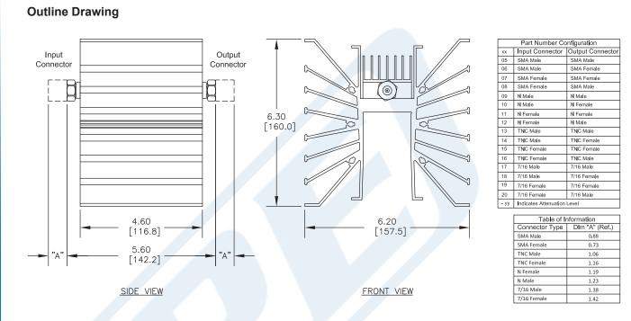
30 dB Fixed Attenuator, N Female To N Male Directional Black Aluminum Heatsink Body Rated To 300 Watts Up To 3 GHz from Pasternack Enterprises has same day shipment for domestic and International orders. Our RF, microwave and millimeter wave products maintain a 99% availability and are part of the broadest selection in the industry.
