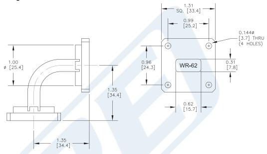
WR-62 Waveguide E-Bend with UG-419/U Flange Operating from 12.4 GHz to 18 GHz from Pasternack Enterprises has same day shipment for domestic and International orders. Our RF, microwave and millimeter wave products maintain a 99% availability and are part of the broadest selection in the industry.
