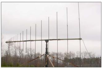
and a +20 degree elevation tilt. An optional dielectric mast with provision for tower mounting is available. The mast breaks into 2 pieces 10 foot long.
