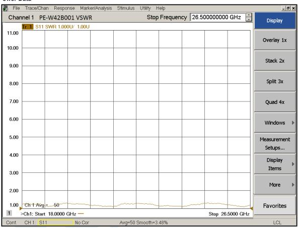
Click the following link (or enter part number in "SEARCH" on website) to obtain additional part information including price, inventory and certifications: WR-42 Instrumentation Grade Waveguide E-Bend with UG595/U Flange Operating from 18 GHz to 26.5 GHz PE-W42B001
