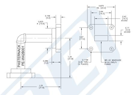
WR-42 Instrumentation Grade Waveguide E-Bend with UG595/U Flange Operating from 18 GHz to 26.5 GHz from Pasternack Enterprises has same day shipment for domestic and International orders. Our RF, microwave and millimeter wave products maintain a 99% availability and are part of the broadest selection in the industry.
