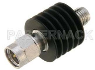
10 dB Fixed Attenuator, SMA Male To SMA Female Aluminum Heatsink Black Anodized Body Rated To 5 Watts Up To 18 GHz
