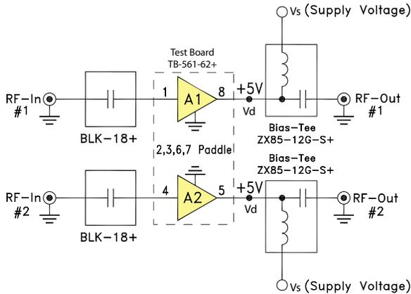
**Fig 1a.** Block Diagram of Test Circuit used for characterization. (DUT tested in Mini-Circuits Test board TB-561-62+, except for IP2). Gain, Return loss, Output Power at 1dB compression (P1 dB), output IP3 (OIP3) and noise figure measured using Agilent’s N5242A PNA-X micro-wave network analyzer.
