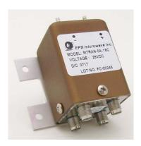
The M version Transfer (MTRAN) is a four port switch with two independent pairs of RF paths. These pairs are actuated simultaneously. This actuation is similar to that of a double-pole-double-throw switch. Failsafe and latching switching modes are available. Other options include position indicator contacts and choices of connectors. See Model Numbering System for other options.
