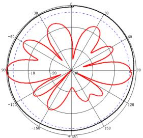
Freq:928MHz Date:2014-04-01 Elevation:H-plane Polar-Across:Main Polarization:Vertical Max:-8.26dB H-PBW(3dB):360.00° FBR:0.59dB
