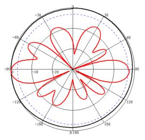
Freq:914MHz Date:2014-04-01 Elevation:H-plane Polar-Across:Main Polarization:Vertical Max:-8.24dB HPBW(3dB):360.00\* FBR:0.53dB
