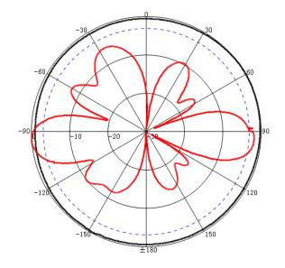
Freq:900MHz Date:2014-04-01 Elevation:H-plane Polar-Across:Main Polarizion:Vertical Max:-8.06dB HPBW(3dB):360.00\* FBR:0.36dB
