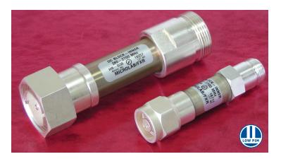
The Microlab HR-20 series DC Blocks are used to prevent the flow of direct current and low frequency current surges along the inner conductor of a transmission line, while permitting the unimpeded flow of RF signals. Applications include the blocking of current surges in subway tunnels, at antenna sites during lightning storms and to route DC to tower mounted amplifiers.
