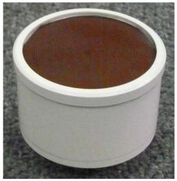
very good candidate for electronic-warfare, direction-finding, telemetry and surveillance systems, as well as flush-mounted airborne applications. The antenna can be used as a broadband feed for reflector antennas. The RF output of the antenna is a type SMA female connector, located at the bottom of the antenna. The antenna is rated for 1 Watt of input power.
