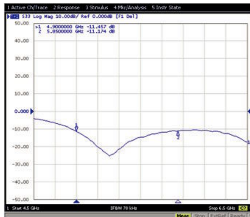
Antenna S11 on Test Board
