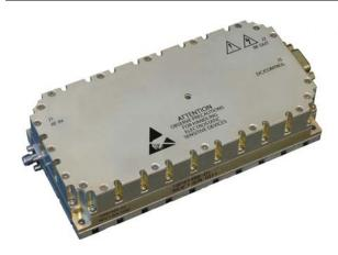
Comtech PST has announced the release of a solid state Class "AB" linear amplifier which operates over the full 2500-6000 MHz frequency band and delivers a minimum of 20 watts. The amplifier uses the latest Gallium Nitride (GaN) technology and is housed in a relatively small package measuring only 6.4" x 3.125" x 1.5" (excluding connectors). Features include temperature monitoring through digital interfacing.
