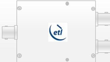
COM02L1P-2562 is a 2-way passive L-band splitter/combiner with 10MHz and DC pass from both output ports to the common port and DC block between outputs.
