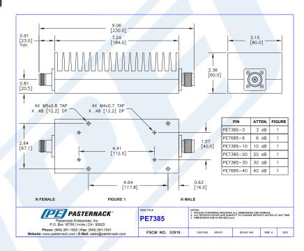
20 dB Fixed Attenuator, N Male To N Female Black Anodized Aluminum Heatsink Body Rated To 100 Watts Up To 3 GHz from Pasternack Enterprises has same day shipment for domestic and International orders. Our RF, microwave and millimeter wave products maintain a 99% availability and are part of the broadest selection in the industry.
